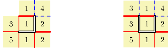
Figure 15: Crease pattern around an L-slit (left) and a U-slit (right). Numbers indicate the face of the six-sided die in the folded state; thinner lines denote creases folded by \pm 90^\circ ; thicker lines denote creases folded by \pm 180^\circ ; mountain folds are drawn solid/red; and valley folds are drawn dashed/blue.
