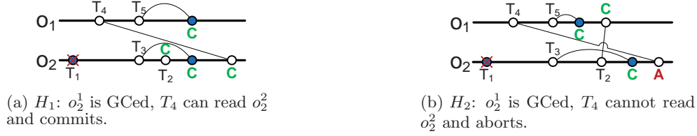
Figure 4: H_1 and H_2 are indistinguishable if a read-only transaction T_2 does not leave any trace after its execution.
