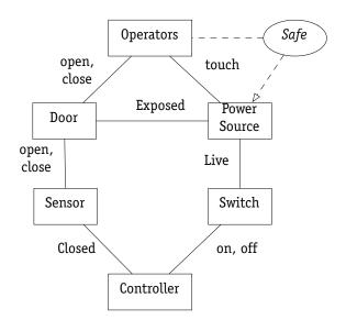
(The requirement is shown as an oval, with arcs to the domains whose phenomena are mentioned in the requirement. An arc with an arrow identifies a domain that will be constrained by the requirement.)
