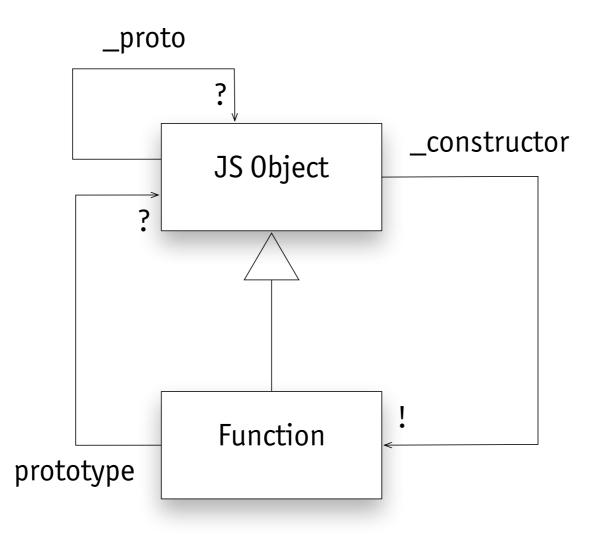
**all** o: JSObject | o.\_proto = o.\_constructor.prototype
