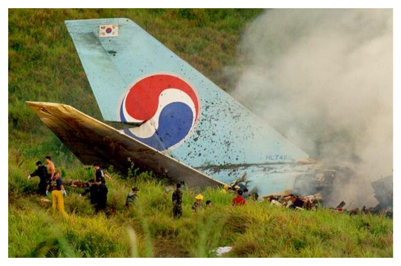
If the ARTS IIA minimum safe altitude warning system had been operating as initially intended, a visual and aural warning would have activated about 64 seconds before flight 801 impacted terrain --NTSB report
