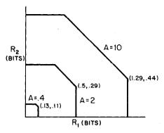
Fig. 6. Achievable rate region as function of signal/noise A.
