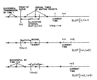
Fig. 12. Record of collision resolution period for FCFS splitting algorithm.
