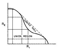
Fig. 5. Achievable rate region for collision channel.
