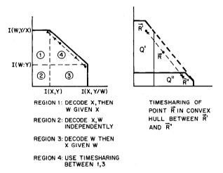
Fig. 9. Timesharing construction to obtain any achievable rate pair without joint decoding.
