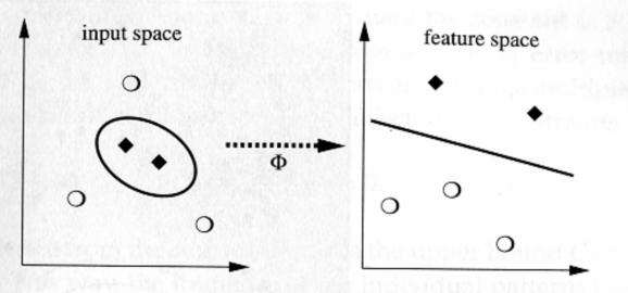
**Figure 1.6** The idea of SVMs: map the training data into a higher-dimensional feature space via  $\Phi$ , and construct a separating hyperplane with maximum margin there. This yields a nonlinear decision boundary in input space. By the use of a kernel function (1.2), it is possible to compute the separating hyperplane without explicitly carrying out the map into the feature space.
