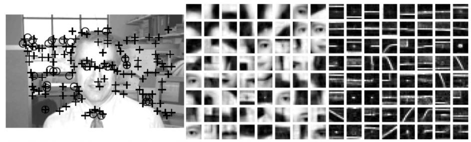
**Fig. 3.** Points of interest (left) identified on a training image of a human face in cluttered background using Förstner's method. Crosses denote corner-type patterns while circles mark circletype patterns. A sample of the patterns obtained using k-means clustering of small image patches is shown for faces (center) and cars (right). The car images were high-pass filtered before the part selection process. The total number of patterns selected were 81 for faces and 80 for cars.
