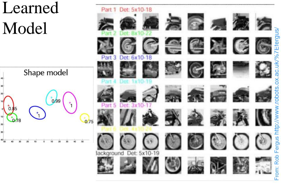
The shape model. The mean location is indicated by the cross, with the ellipse showing the uncertainty in location. The number by each part is the probability of that part being present.
