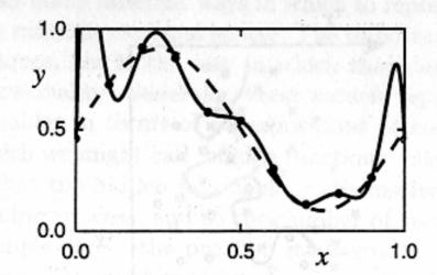
Figure 1.8. The result of fitting the same data set as in Figure 1.6 using a 10thorder (M = 10) polynomial. This gives a perfect fit to the training data, but at the expense of a function which has large oscillations, and which therefore gives a poorer representation of the generator function h(x) than did the cubic polynomial of Figure 1.7.
