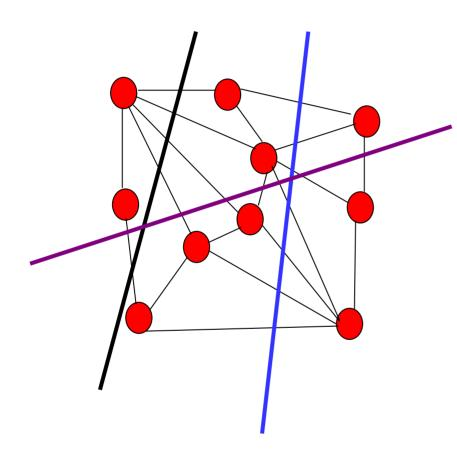
A cut of a graph *G* is the set of edges *S* such that removal of *S* from *G* disconnects *G*.
