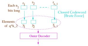
Alg: Decode Meaches ymbol of inner code by Brute force. Then decode the "received word" corr. to outer code.
