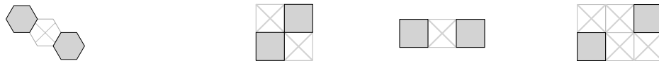
■ Figure 3 Forbidden patterns in previous algorithms for hexagonal and square pivoting modules
